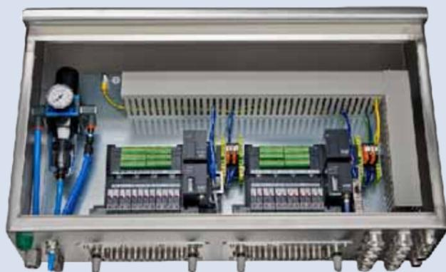
*The hygienic design pneumatic housings are available in 3 standard widths at constant constructional height and depth. This enables a flexible adaption, enclosures standing shoulder-to-shoulder in close proximity of the valve nodes - and thus installed right in the middle of the hygiene-sensitive process field.*
